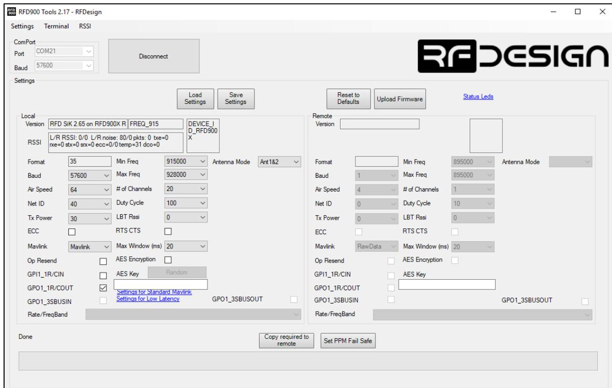
Figure 8 – Vehicle modem configuration on RFD900 tools.
