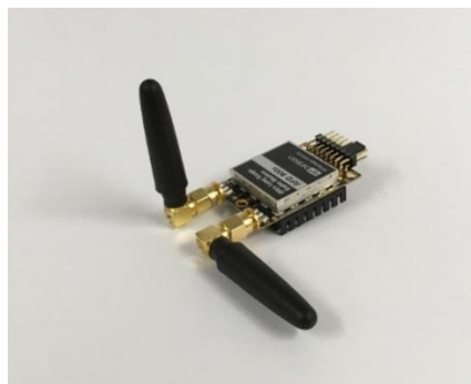
Figure 8-1: Antenna configuration to achieve polarisation diversity
