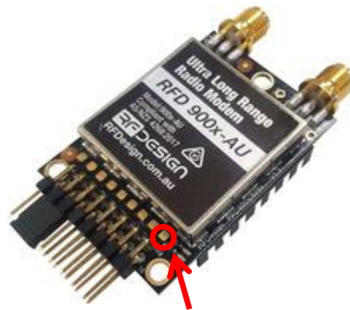
Figure 4-2: Boot mode pad
