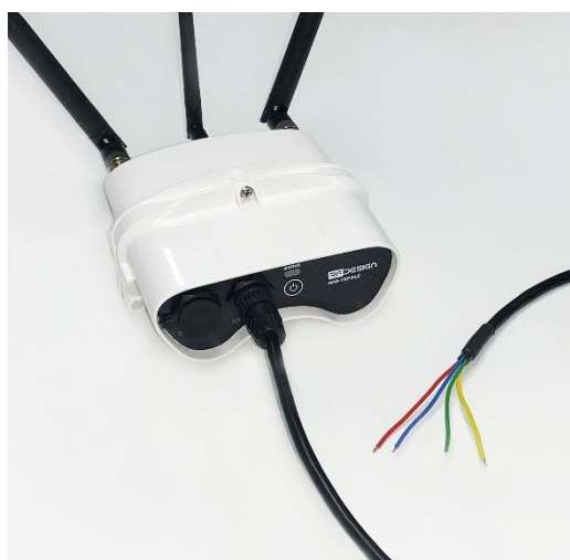
Figure 2 - Power connection: red VCC, blue GND, green BUTTON- and yellow BUTTON+
