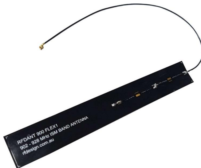
Figure 21: RFD Flex1 antenna with 300mm cable
