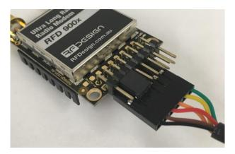
Figure 3-1: An FTDI cable connected to the RFD900x modem
