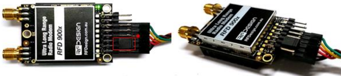
Figure 13 - Modem connected to FTDI cable (pins 1,3,5,7,9,11) to enable serial communications. *Jumper connection (pins 4&6).
